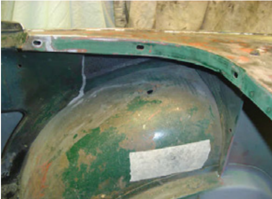
Fig 4 Masking off the wheel arch for marking.
