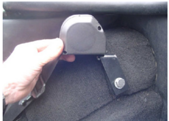
Fig 9 Final Installation NB Inertia Mechanism mounted horizontally
