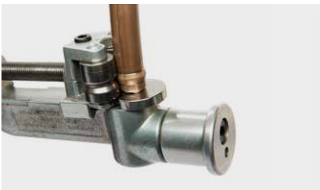
Picture 5 Lubricate inside and outside of the tube, turn with slightly applied pressure
