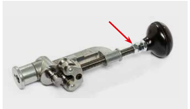
Picture 6 If many similar beads are to be made, lock the stop nuts on the adjusting screw
