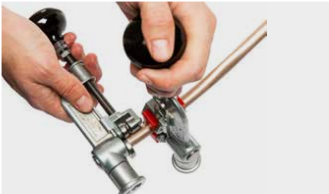
Picture 5 Lubricate inside and outside of the tube, turn with slightly applied pressure
