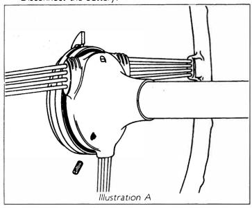
Your old control head is secured to the steering wheel by three grub screws located in the hub of the steering wheel (Illustration A). These may be rusty. If they are, use penetrating oil on the screws before attempting to remove them. The screws are slotted, so care should be taken not to destroy the heads.
