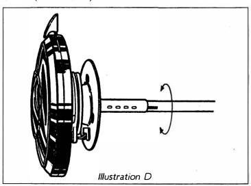
The control head has a short stator tube attached to it (Illustration D). This tube fits over the longer stator tube that goes down through the steering column. The short tube has indents that fit into a slot in the longer tube. The longer tube may have to be rotated to allow for proper alignment of the control head.
