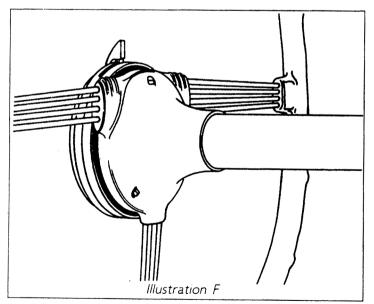
Secure the control head to the steering wheel hub by tightening the grub screws. If you tighten one screw down too much, the control head will become cocked and the rest of the screws will not catch the mounting
