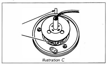
Check that the alignment of the turn signal control lever is opposite of the canceling mechanism. When installed in the car, the lever should be in the 12 o'clock position, and the canceling mechanism should be at 6 o'clock (Illustration C).
