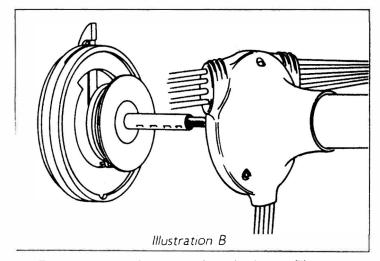
The control head can now be withdrawn (*Illustration* 3). It will probably be necessary to feed the bullet ends on the harness into the stator tube where it extends out of the bottom of the steering box.
