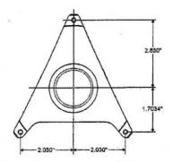
Figure 2: Bolt pattern of the Tri-Lite assembly
