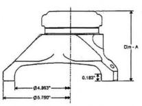
Figure 3: Side-view of Tri-Lite assembly
