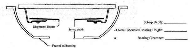
Figure 1: Set-up Depth Measurement
