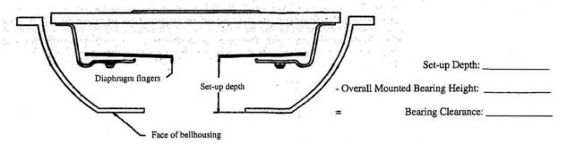
Figure 1: Set-up Depth Measurement
