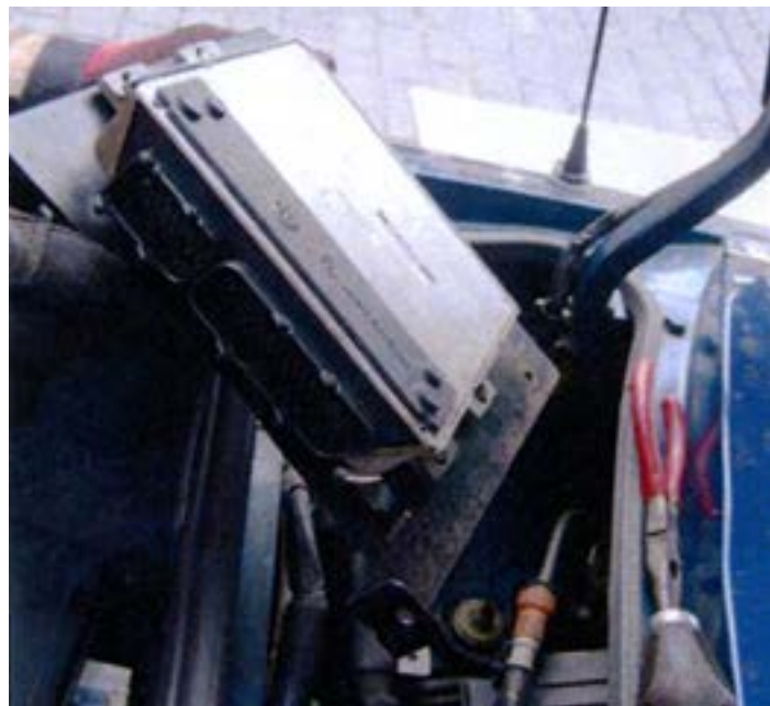
Figure 22: The ECU needs to be moved.
