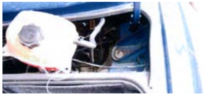
Figure 15: Move the coolant expansion tank.
