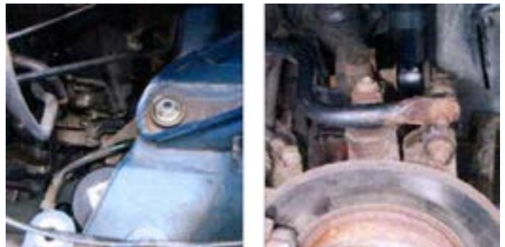
Figure 19-20: The upper nut torque is 50Nm reconnect the rear anti roll bar, torque 45Nm.
