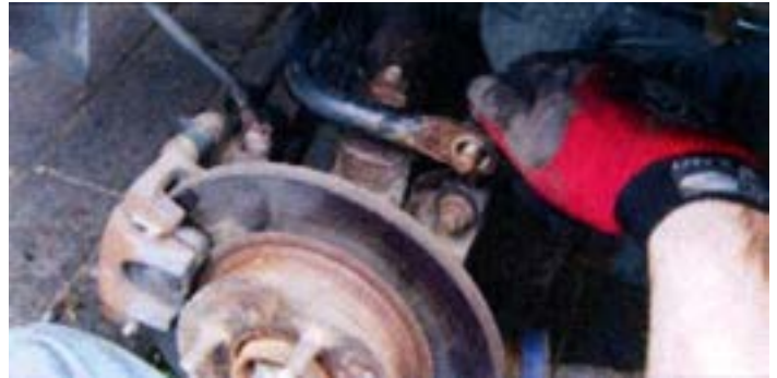
Figure 16: Undo and remove the anti roll bar to link top nut and bolt.
