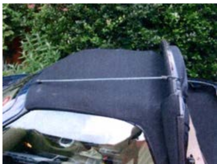
Figure 24: Hold spar in position.
