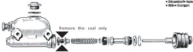
Note: Remove the valve rubber only from this check valve. Leave the metal body in place
