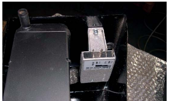
11. Select positive or negative wiring diagram to suit vehicle earth configuration. Make connections to the resistor and motor as per correct electrical diagram.
