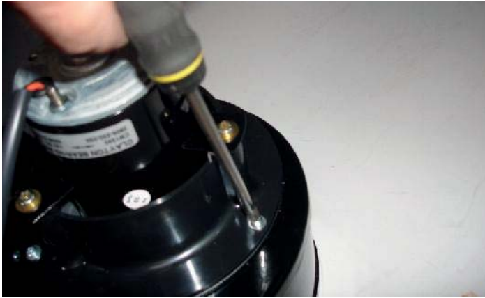
9. Slide fan wheel onto shaft and secure in place through hole drilled in the side of the volute. Accurately position fan wheel so it sits slightly above fan wheel aperture, and tighten grub screw. (Ensure fan wheel sits slightly inside the scroll and does not come into contact with the heater case).
