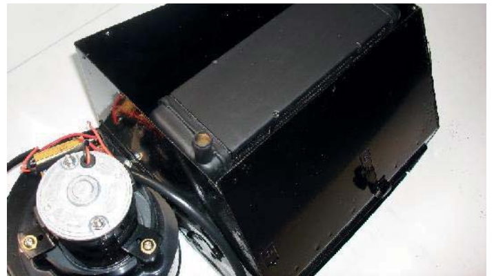
10. Mount resistor to the inside of the heater case into pre-drilled fixing holes.
