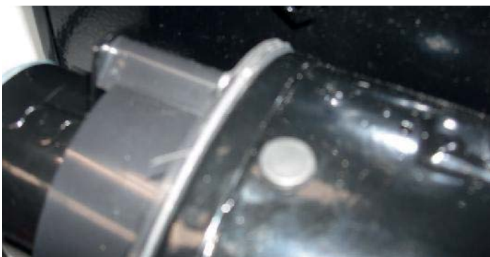
10. Insert rubber blanking grommet into 10mm hole.
