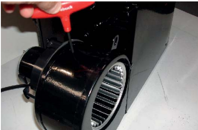
10. Insert rubber blanking grommet into 10mm hole.
