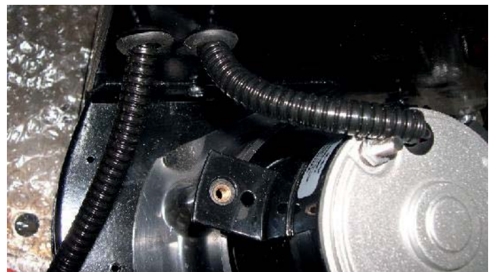
11. Select positive or negative wiring diagram to suit vehicle earth configuration. Make connections to the resistor and motor as per correct electrical diagram.
